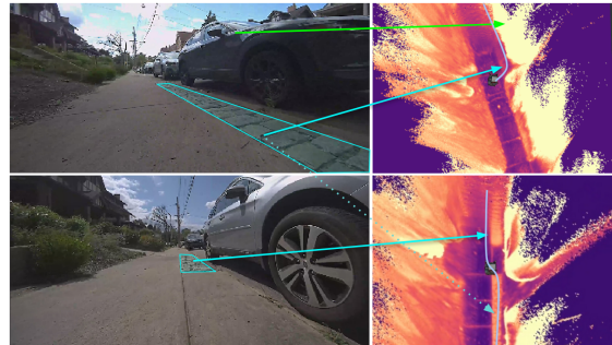
Fig. 8: Evaluation on urban wheelchair: After driving over rough cobblestone, the system quickly recognizes within 5 seconds that it is much rougher than the smooth sidewalk.
